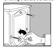
Remove the polystyrene base, set the machine upright and unscrew the two remaining rear bolts.
